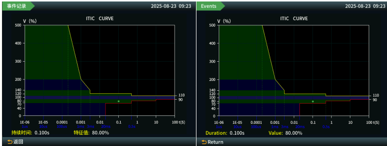
Figure 3-7 ITIC Voltage Tolerance Curve
