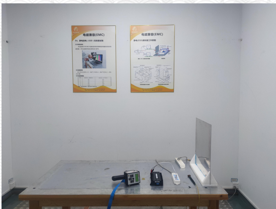
Figure 6: Electrostatic Discharge Test Setup
